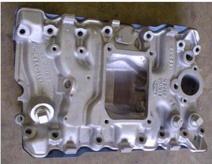
Ported carb/CFI style intake manifold with billet aluminum carburetor adapter and 1" phenolic spacer, list $800, SPECIAL: $400
