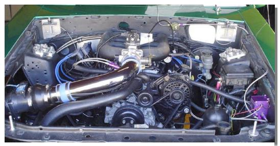
As performance levels increase, so does the maintenance. With our 4.3, we make most of our power naturally aspirated on motor abne. In conjunction with the simple nature of the ZEX nitrous system as our power adder, we have a clean neat engine compartment which simplifies maintenance. No hassles with intercoolers, turbo oil control, piping interference, supercharger belt slip, etc—just clean, simple power.
