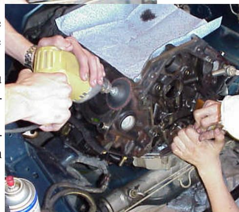
Before we start reassembly we need to transfer some stuff from the old parts to your new stuff. It's a few things on the upper intake, like the throttle body, EGR vacuum valve, PCV line with PCV valve attached. Some stuff on the lower like the coolant bypass fittings and the sensors.
