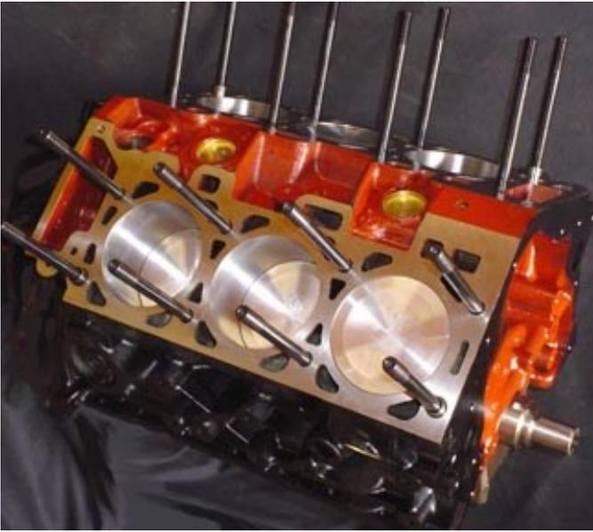
**4.0 SOHC shortblocks** include custom Wiseco forged pistons and rings, new race prepped forged rods, ARP head studs, new rod bolts, new Ford crank, bearings, freeze plugs, and seals. Each shortblock is cleaned and inspected, aligned, decked, bored, torque plate honed, glyptaled, balanced, and professionally assembled.
