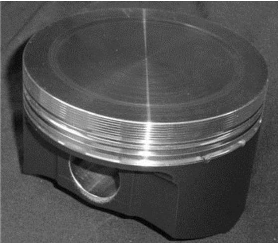
Boost or nitrous kills stock 4.0 hypereutectic pistons because the top ring land is too close to the crown for power adder applications. **Wiseco piston kits** are made to our specs featuring many durability improvements for boost and nitrous applications:
