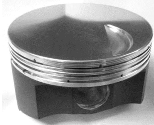
**Our forged piston kits** are made to our specs by Wiseco. Our forged pistons include stronger and thicker stronger crowns and skirts, generous ring lands. Most include off-set pins for reduced wear and quieter operation. Fits all 3.8s, 3.9s, 4.2s, "Long Rod" 4.3 strokers, SuperCoupes.
