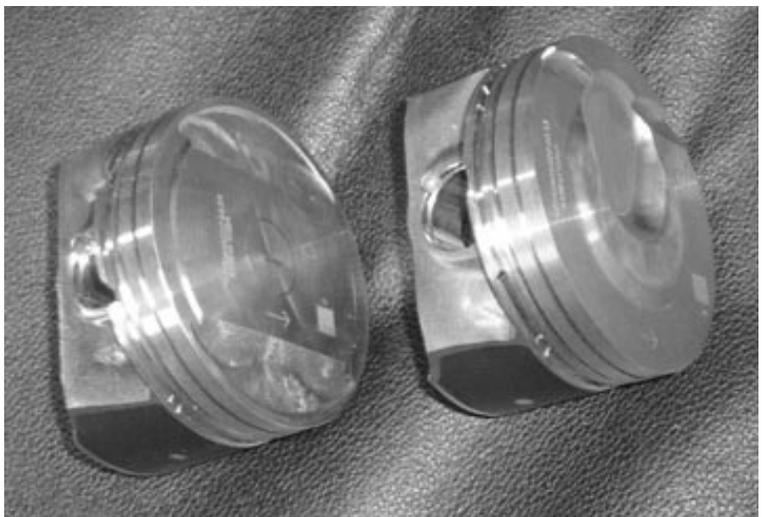
The pistons of the EcoBoost and the generic 3.5/3.7 are both hypereutectic and use anti-friction coated piston skirts, this has become the norm for modern production engines. The pistons are made with internal lightening pockets to reduce reciprocating weight and use modern thin, high performance rings with a Dykes or Napier-style 2nd ring. The pistons are light weight at 372 grams but the wrist pins are thick walled and pretty heavy at 119 grams. The EcoBoost piston
