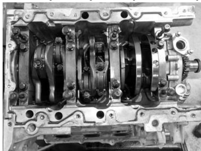
skirt. Like other modern engines, the Cyclone uses a removable rear main seal cover plate and a structural rear sump cast aluminum oil pan. The cylinders feature cast-in liners and are fully floating at the top of the block.
