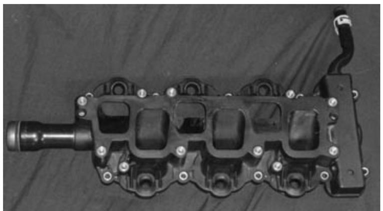
The 3.5 uses an aluminum lower intake manifold with equal sized ports but of similar shape, again, porting will be beneficial and yield a better transition to the oval intake port shape in the cylinder head. The 3.5 aluminum lower intake manifolds have different bolt and coolant transfer ports and will not interchange with the 3.7 lower intakes.
