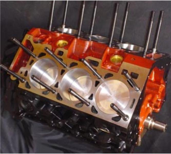
**4.0 SOHC shortblocks** include custom Wiseco forged pistons, race prepped stock forged rods, ARP 2000 head studs, new rod bolts, polished crank, seasoned SOHC block, rings, bearings, freeze plugs, and seals. Each shortblock is cleaned and inspected, aligned, decked, bored, torque plate honed, glyptaled, balanced, and professionally assembled.
